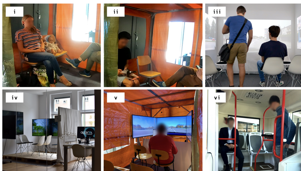
Figure 2. Examples of static interior mock-ups of (shared) AVs in combination with other prototyping methods. Images (i,ii) were taken from Schuß et al. [40], who used a tent-based setup in combination with a dynamic enactment simulation and physical items. Images (iii–v) show video-based simulation setups with different spatial mock-up components (chairs, walls, tent, whiteboard, wooden pellets) [10,30,46]. Image (vi) shows a high-fidelity interior of a shared AV.
