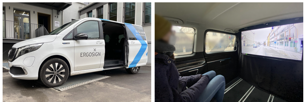
Figure 5. Example of a video-based Wizard-of-Oz setup that we created for our in-vehicle interaction studies [44] inspired by the works of Karjanto et al. [66] and Detjen et al. [42].
